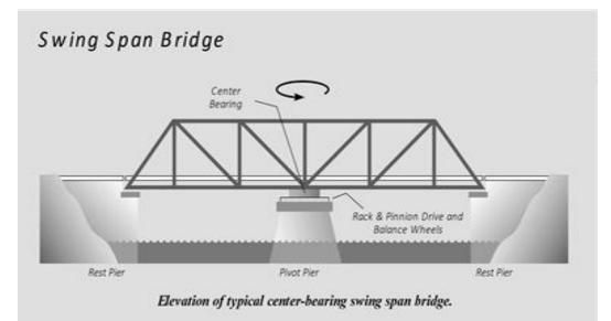
Fig.1.Elevation of Swing Span Bridge
